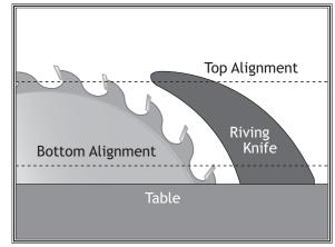
**Figure 100.** Checking riving knife-to-blade alignment.
